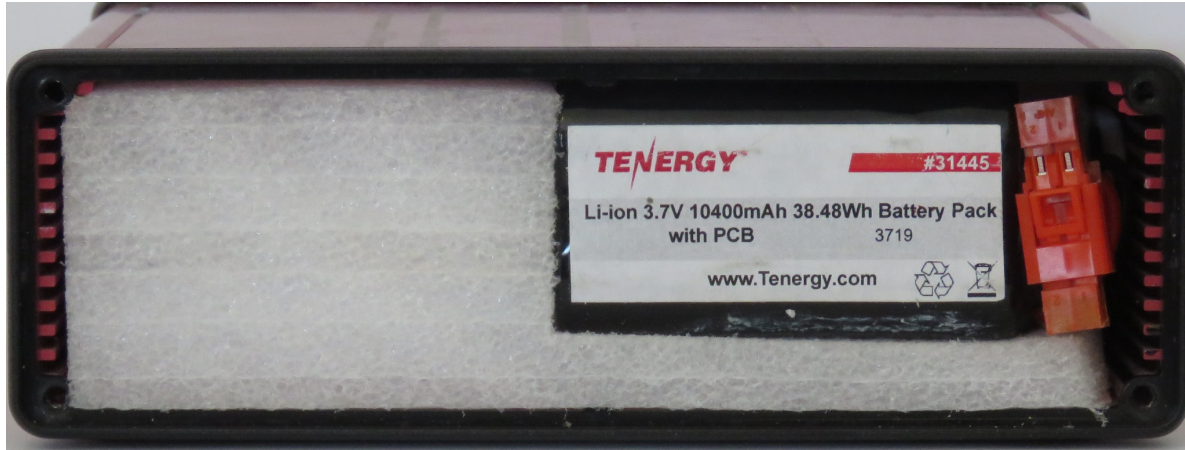
TKMD Backup Battery (Battery Access Cover Removed)
