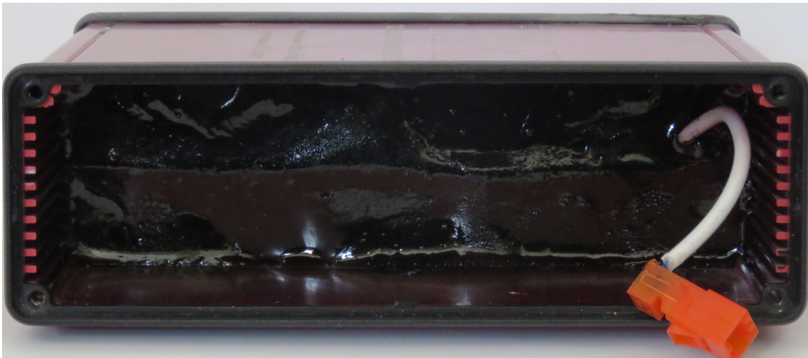
TKMD Epoxy Potting (Battery Access Cover, Support Foam and Battery Removed)
